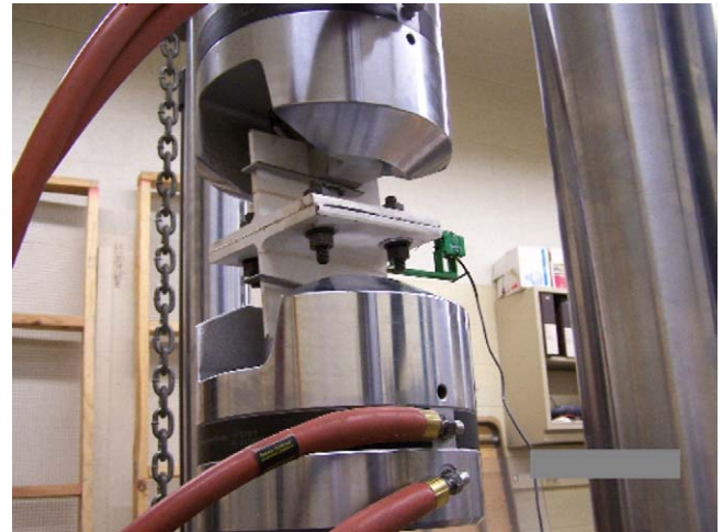
Fig. 8. A photograph of a typical t-stub test set-up.
