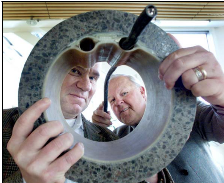
Figure 13 -- Cables in a Liner
