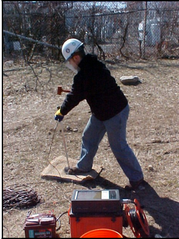
Figure 5 -- Installation of Surface Geophones
