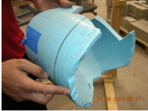
Figure 19: Pipe Piece after Failure of Specimen 3
