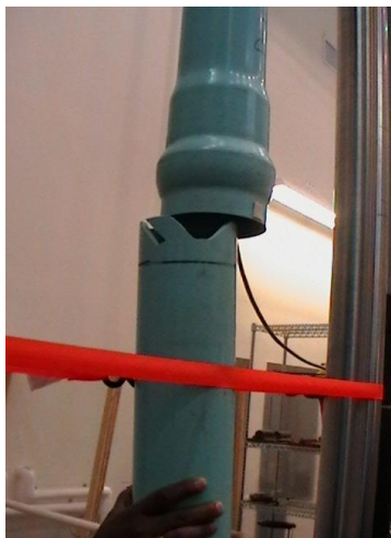
Figure 12: Failure of Specimen 2
