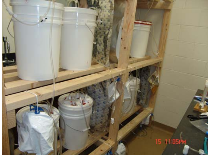
Figure 1 Simulation of Bioreactor Landfill in the Laboratory
