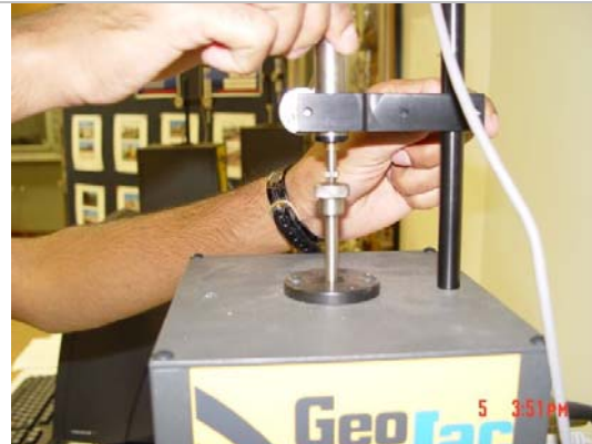
Adjust the displacement LVDT
