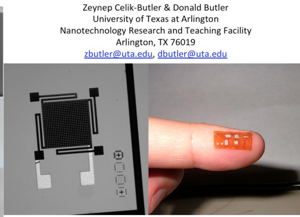
(left) An optical micrograph of a z-axis accelerometer fabricated on a polyimide substrate. (right) A flexible polyimide die containing six z-axis and lateral axis accelerometers, conformally resting on a finger.
