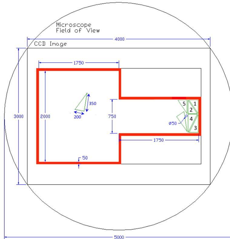
Figure 4: Arena Dimensions for the Microassembly event
