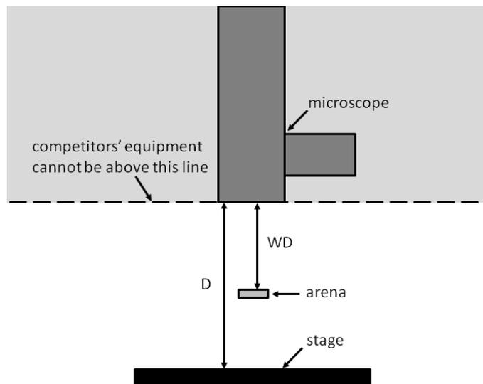
**Figure 5: Front view schematic of the microscope and microscope stage**
