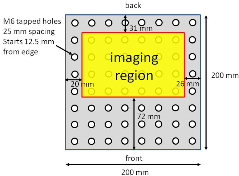
**Figure 6: Top view schematic of the microscope stage with a highlighted area indicating the region in which samples can be imaged**
