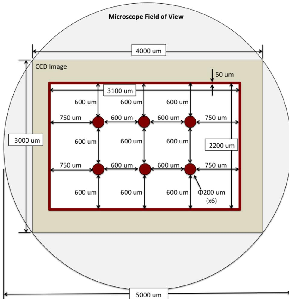
**Figure 1: Arena Dimensions for the Autonomous Mobility Challenge (note: 3100  $\mu\text{m}$  width should read 3300  $\mu\text{m}$ )**
