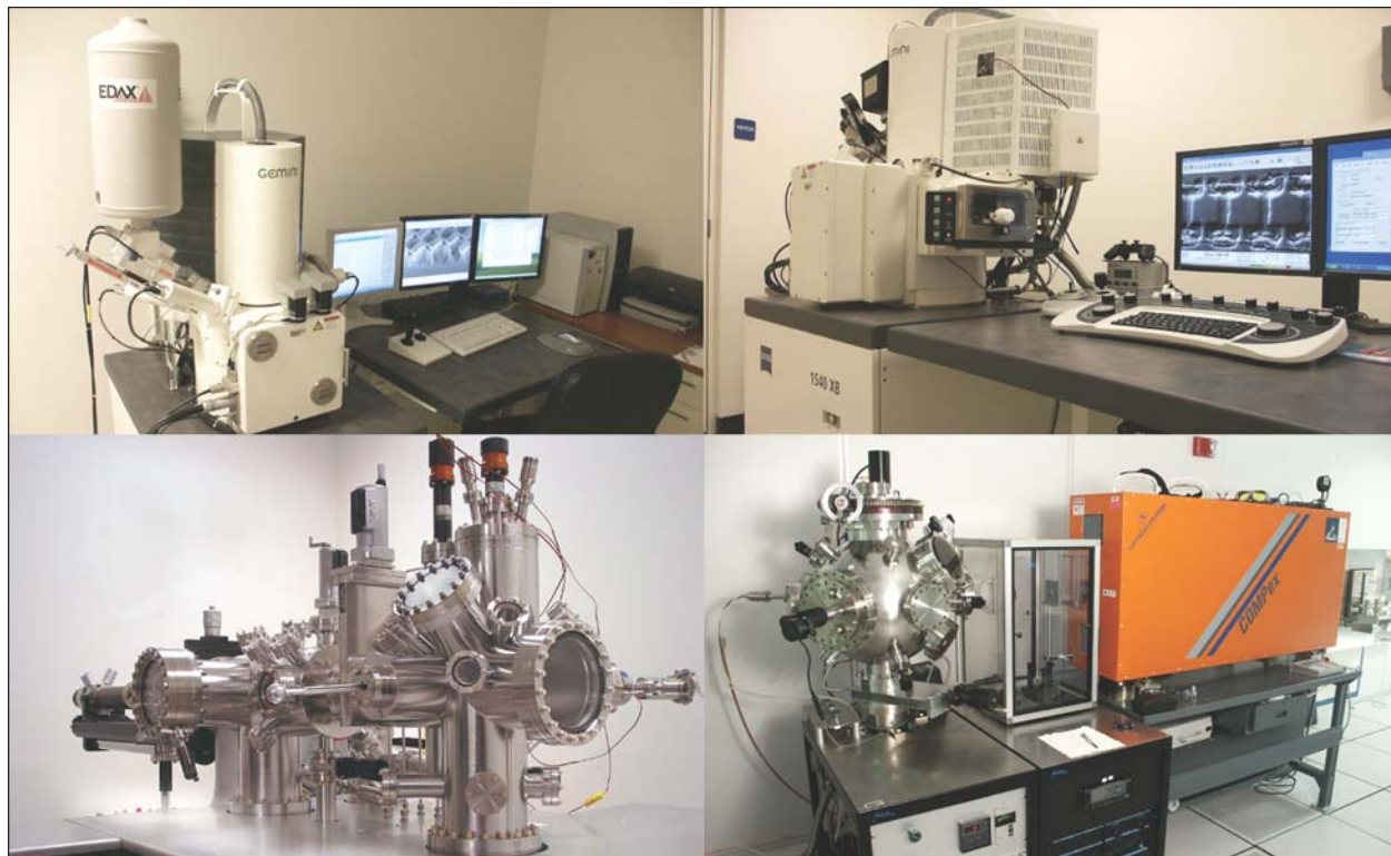
Several pieces of specialized equipment were acquired during the year. Shown above, clockwise from top left: Zeiss 1540XB three-gas, Focused Ion Beam system; Zeiss Supra 55VP Scanning Electron Microscope, capable of sub-nanometer resolution; Neocera turn-key pulsed laser deposition system with 18-inch turbo-pumped vacuum chamber; RHK Ultra-high Vacuum Scanning Tunneling Microscope with surface preparation chamber.
