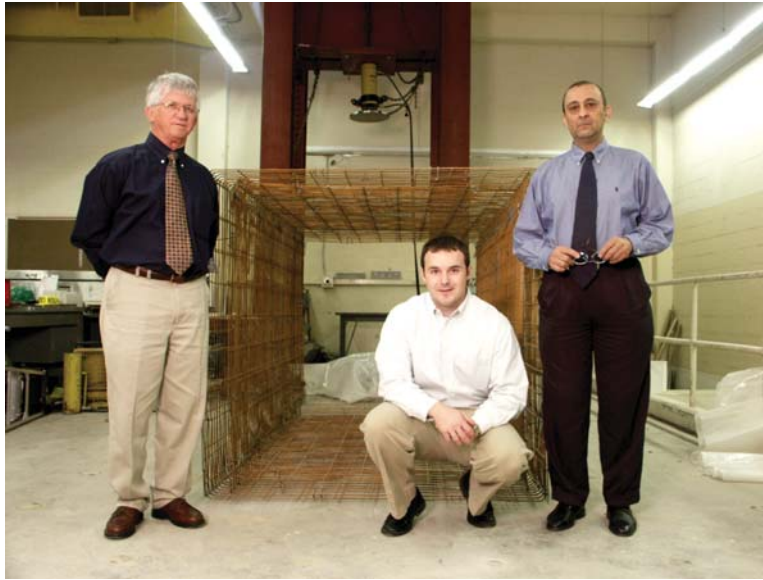
Dr. John Matthys, master's student Jarrod Burns and Dr. Ali Abolmaali examine the reinforcing cage of a concrete box culvert. The team's research in the Structural Engineering Laboratory will use hydraulic rams and a variety of laser sensors to investigate the shear capacity of pre-cast concrete box culverts.
