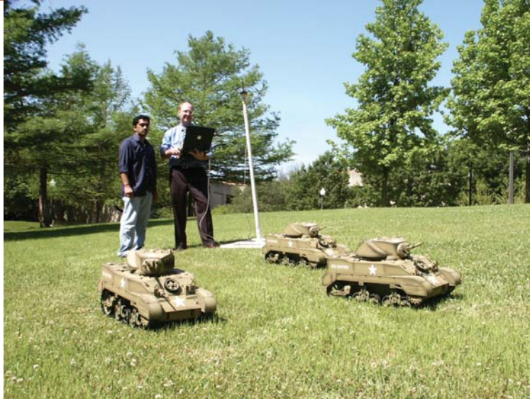
Dr. Brian Huff evaluates a prototype wireless interface designed by master's students Udayakumar Vasudeva (left) and Praveen Kalidindi to support interaction with a team of autonomous ground vehicles. Practical uses of this technology include humanitarian minefield reclamation and the creation of mobile wireless sensor networks and autonomous actuators for a broad range of applications.
