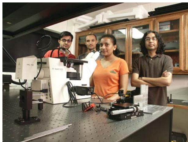
Graduate students Kapil Langer and Manish Kankari and Dr. Digant Dave watch as graduate student Rakhee Subramanyam adjusts an inverted microscope platform, part of a multimodal optical imaging system they are constructing using lasers to detect anomalous tissue and cells and to distinguish normal cells from cancerous ones.
