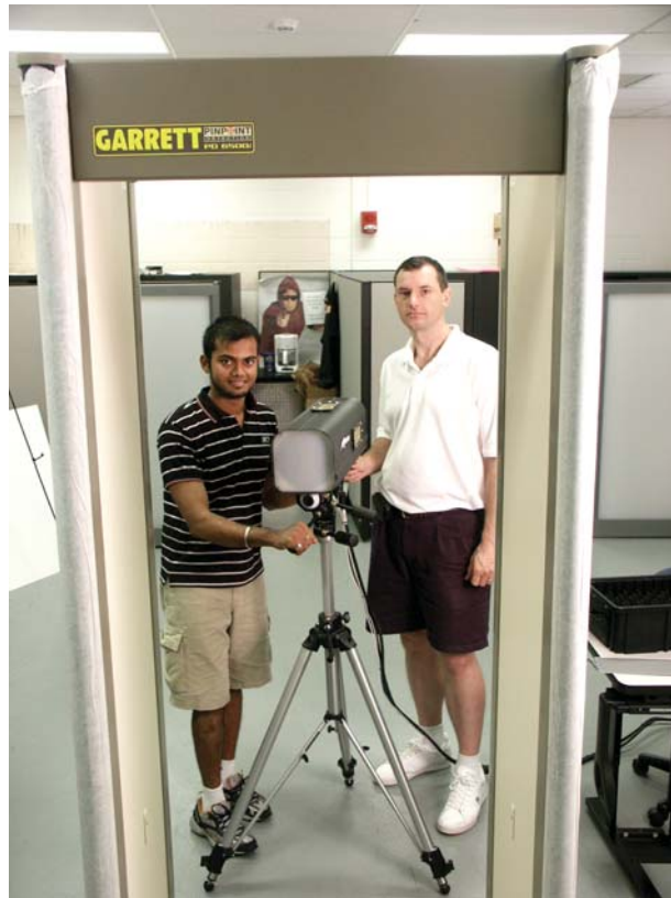
Graduate research assistant Amar Singh and Dr. Larry Holder, principal investigator on the Sentry project, are developing techniques for integrating data from a variety of sensors, including the millimeter-wave camera and multi-zone walk-through metal detector shown here, in order to improve the detection of security threats.
