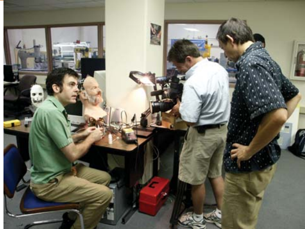
David Hanson of Hanson Robotics demonstrates a lifelike robotic head for a local TV news crew. Hanson developed realistic skin and features for the head and is working with ARRI researchers to improve the servos actuating its facial expressions.
