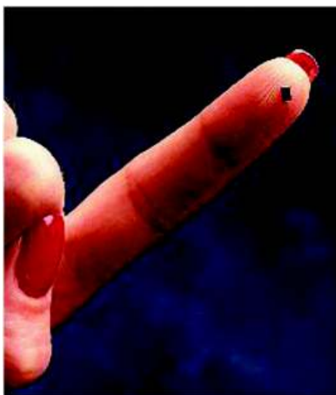
Fig. 1. A medical telesensor capable of transmitting body temperature measurements, indicating the typical size of microfabricated sensors. (From http://ornl.gov/info/ornlreview/rev29_3/text/biosens.htm , accessed 12/31/2008.)
