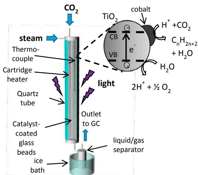
**Fig. 1.** Schematic diagram of photothermal flow reactor with cartoon picture of a single Co/TiO<sub>2</sub> particle undergoing catalysis and TEM picture of cobalt on P25 TiO<sub>2</sub> catalyst.
