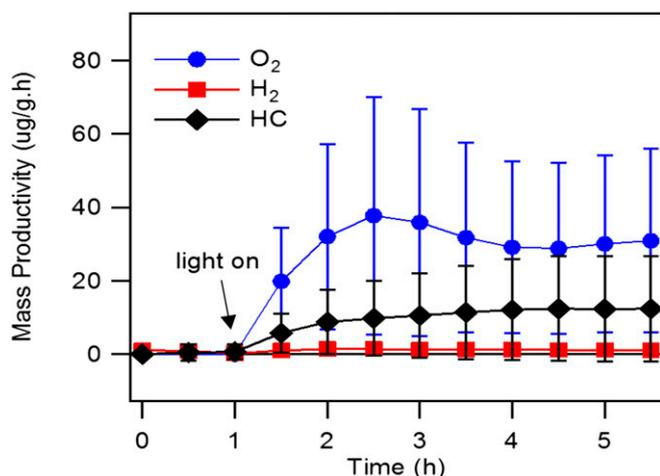
**Fig. 4.** Productivity of O<sub>2</sub> (blue circles) H<sub>2</sub> (red squares), and hydrocarbons (HC) (black diamonds) as a function of time at 200 °C, 6.1 bar, P<sub>H<sub>2</sub>O</sub>/P<sub>CO<sub>2</sub></sub> = 0.6 and 40 sccm.
