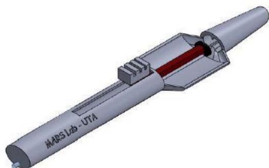
Fig 1. Model of Binocular Injector
