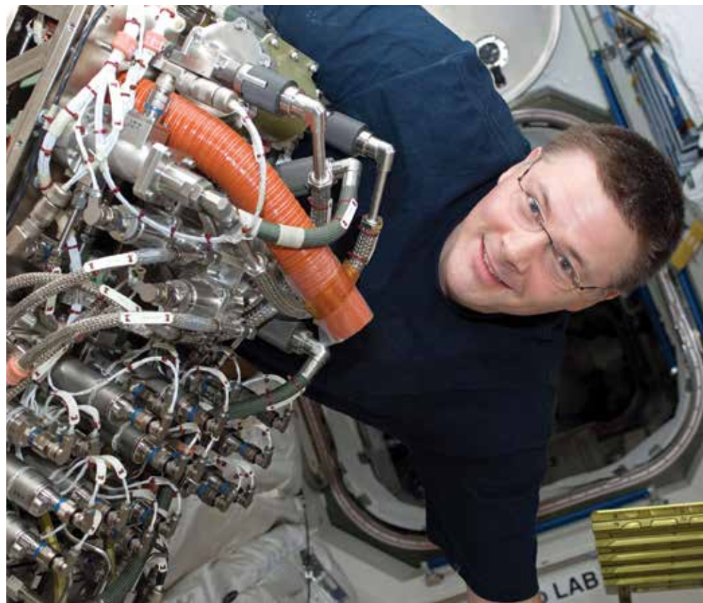
A NASA astronaut with Sabatier, the water creation system of the International Space Station. UTA researchers are working to improve these systems.
