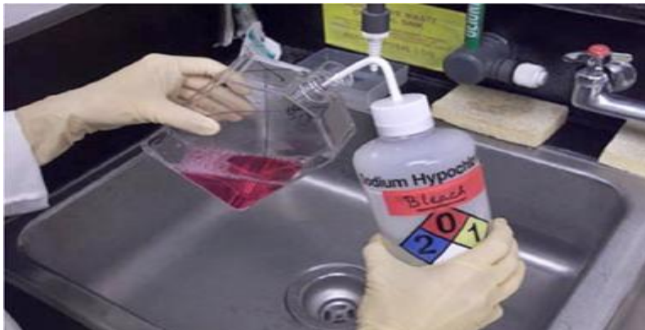
Disinfection of liquid biohazardous waste: A 10% concentration of household bleach in the liquid waste is created.
