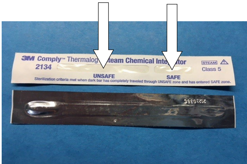
Picture 1. 3M Comply™ Thermalog™ Steam Chemical Integrator (front and back) showing the window marked UNSAFE or SAFE.
