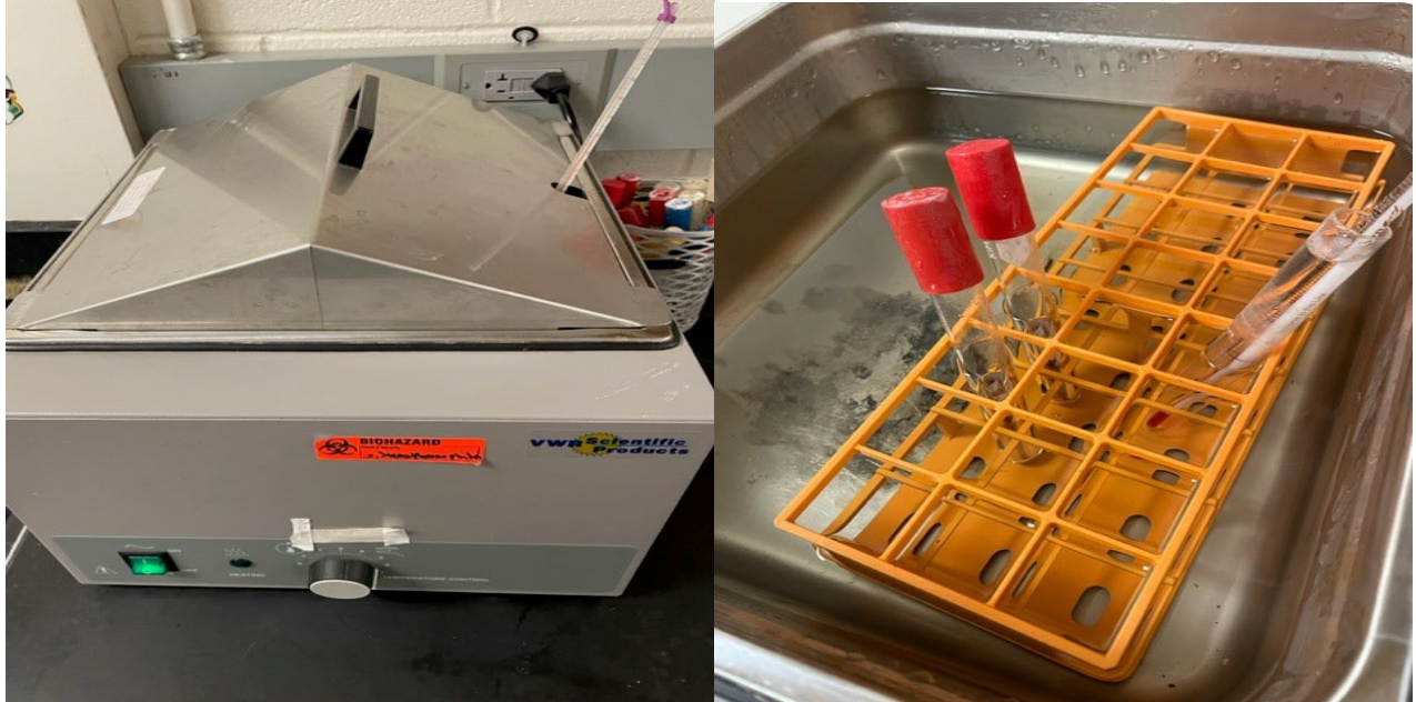
Picture 10 & 11. Biological indicator ampoules in glass test tubes (vertical position) in a water bath
