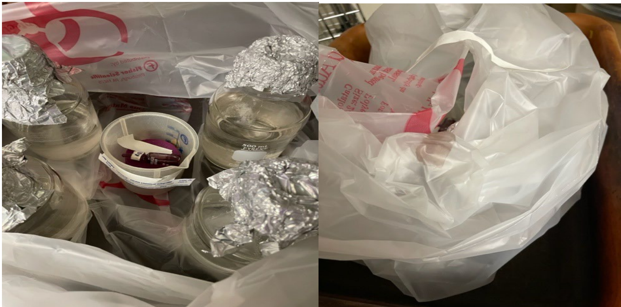
Pictures 8 & 9. The Heat Sink Concept is ready. The autoclavable plastic bag is closed with autoclave tape but left slightly open
