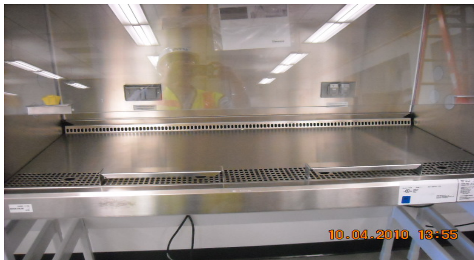
Elbow rests in BSC help to keep airflow steady
