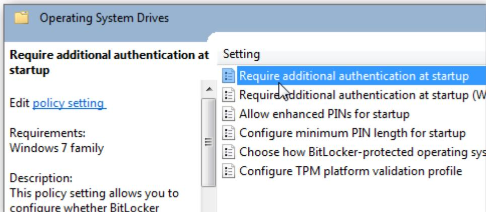
3. Enable the feature and check the box next to Allow BitLocker without a compatible TPM, click Apply and Ok, and close out of Local Group Policy Editor.
