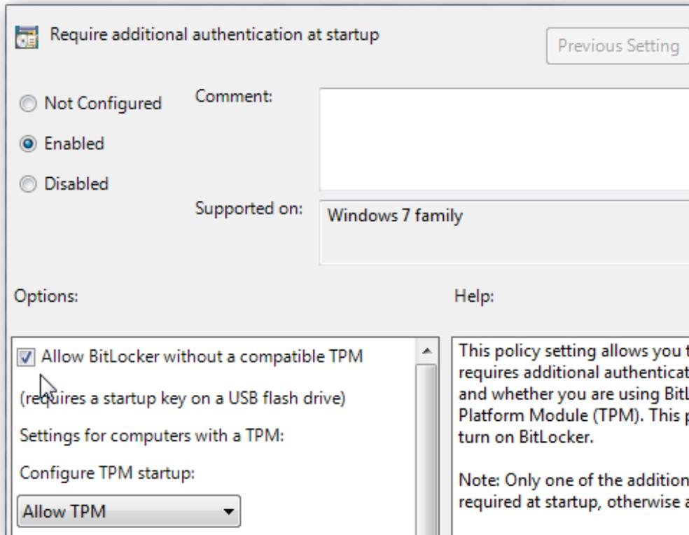
4. Go back to the hard drive you want to encrypt and turn on BitLocker. A restart will be required to prepare the disk, and at this point make sure the flash drive is plugged in. After the restart you're prompted to use the startup key on the flash drive every time you start the computer.
