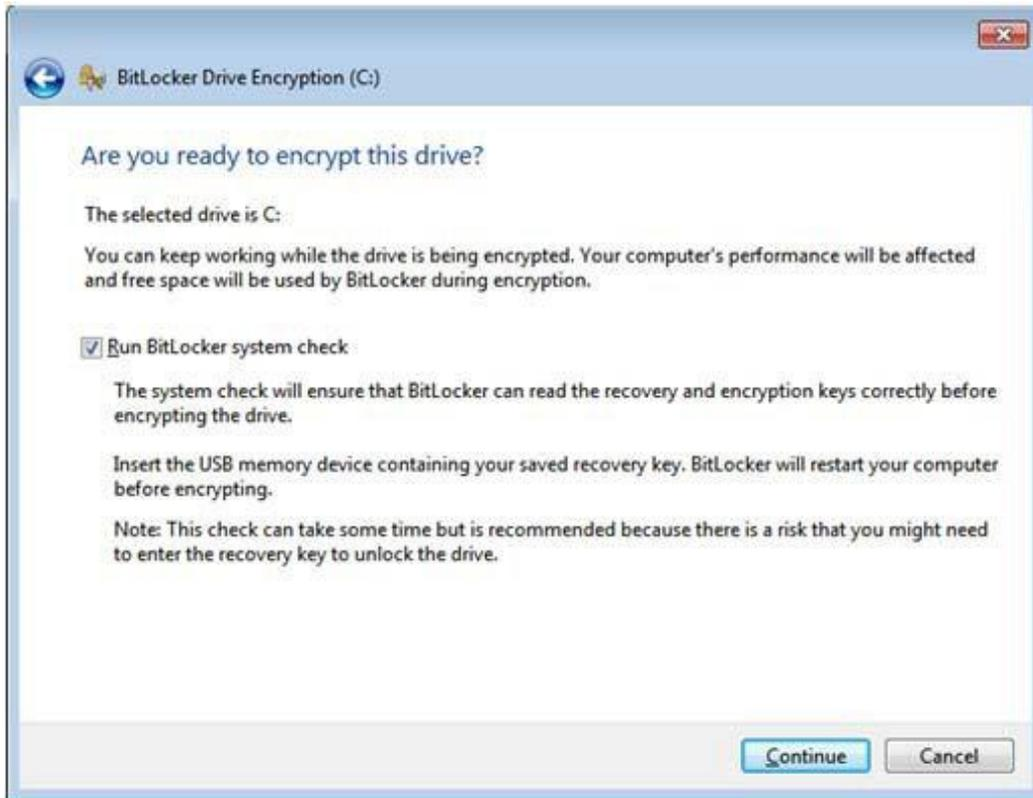
After your computer reboots, windows will begin the encryption process. You can check on the status by going to **Control Panel -> System and Security -> BitLocker**
