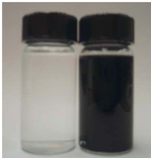
FIG. 1. Typical color of liquids obtained after milling without (left) and with surfactants.
